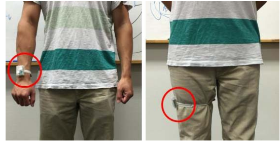
Fig. 5. Inertial sensor placements: right wrist or right thigh.
